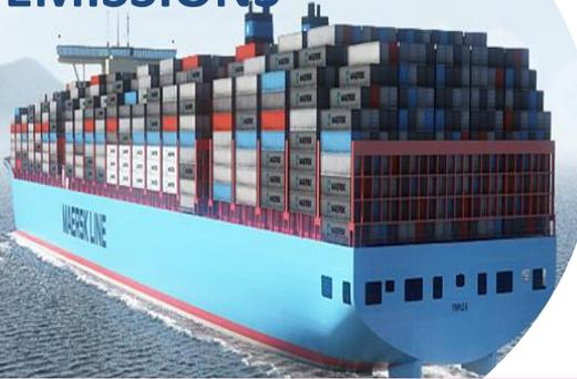
400 meters long, 59 meters wide y 73 meters high, 12.6 meters deep
