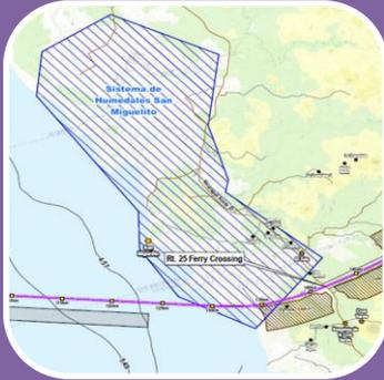
The alignment has been changed to the output from the Lake to the east of the Canal, in order to avoid environmentally sensitive areas.
